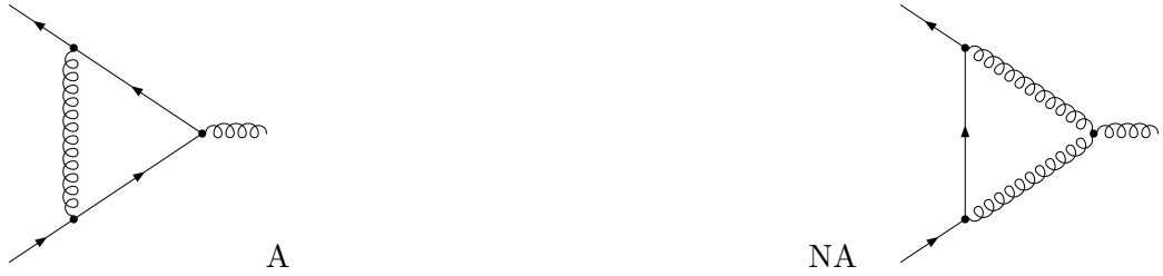
Figure 16: The quark-gluon vertex at one loop. The left diagram labelled A is the Abelian-like term \Gamma_\sigma^A , and the right diagram labelled NA is the non-Abelian term \Gamma_\sigma^{\text{NA}} .
